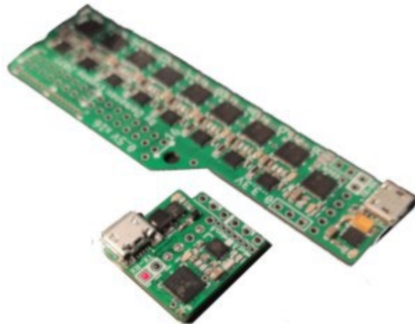
Figure 1: Image of a single MCU read-out board for a 2-channel detector and a 9 MCU board designed for a 16 channel detector.
